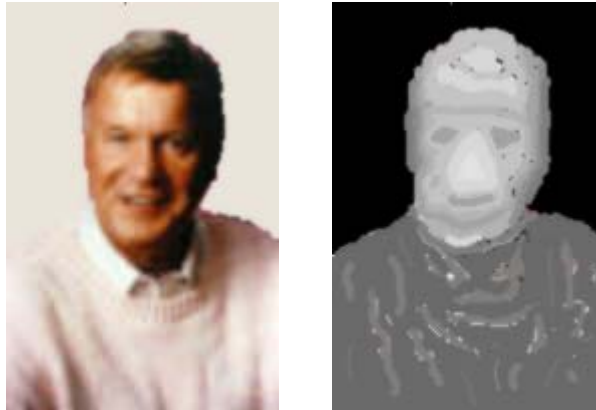
Figure 1. An intensity image and grayscale-coded depth image of a person. Since the background is similar color to the person's shirt, it is difficult for the computer to segment the person from the background using the intensity image. The segmentation is trivial using the depth image.
