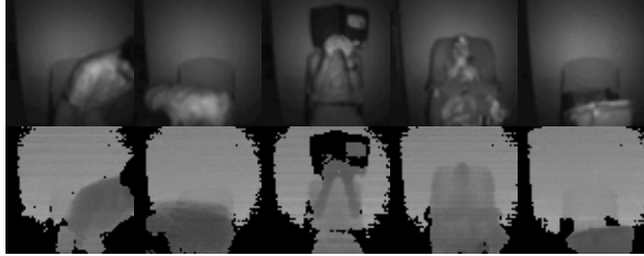
Figure 1. Examples of challenging cases. The first row shows the brightness images, whereas the second row shows the depth images. The depth images are color-coded such that the color becomes darker as the object is closer.
