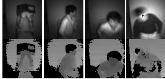
Figure 5. Some failure cases for the algorithm. These cases usually included extreme motion blur, saturation, or extreme configurations of the occupant. There were many similar cases, where the system made a correct classification.
